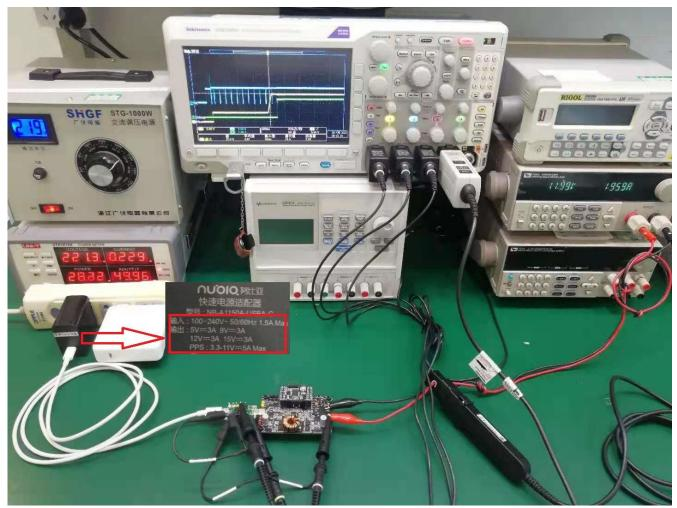
Figure5. 55W PD input, EVB as sink test connection diagram
