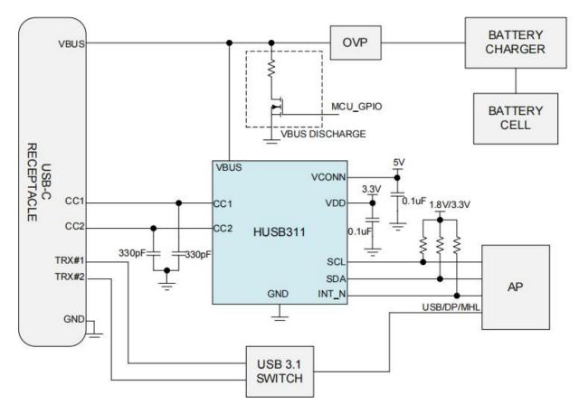
Figure 2. HUSB311 Typical Application Circuit
