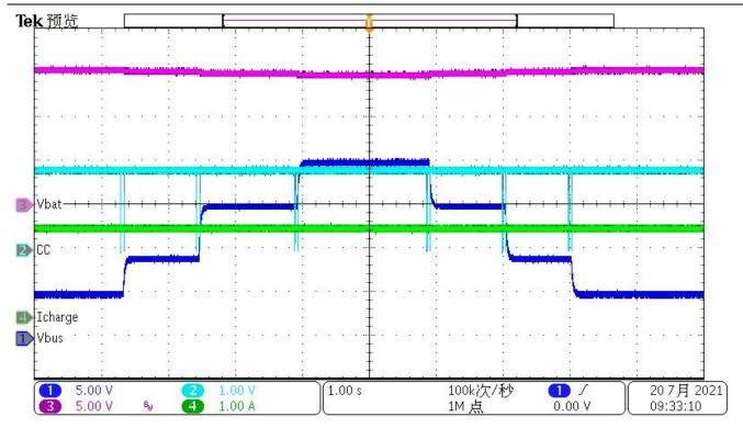
Figure 9. 4 cells battery pack discharging current at 2A with all PDO
