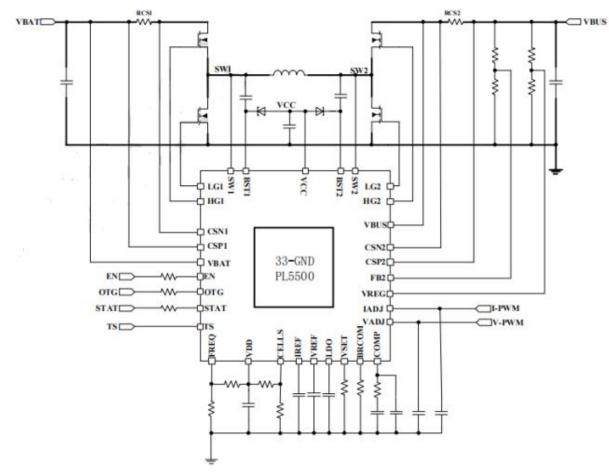
Figure 3. PL5500 Typical Application Circuit
