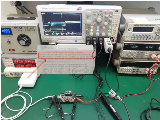
Figure 4. 96W PD input, EVB as sink test connection diagram
